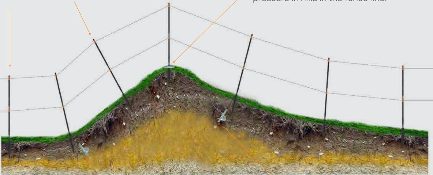
Screw in anchors holding the post down in hollows in the fence line.
