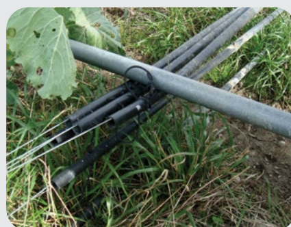
Irrigator wheel assembly half way over the fence line with the irrigator fence deflector bar holding the fence line down.
