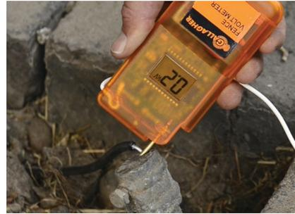
There should be no reading on the Volt Meter; however, up to 200V (0.2kV) is acceptable. If the voltage is higher than this, switch off the Energizer, drive in more earth stakes at the recommended spacings and connect them to the existing earth system until the voltage is down to the acceptable level.
