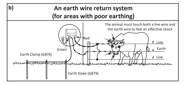
Earth stakes, at least 2m (6ft) long, should be spaced 3m (10ft) apart. Use a minimum of 3 earth stakes.
