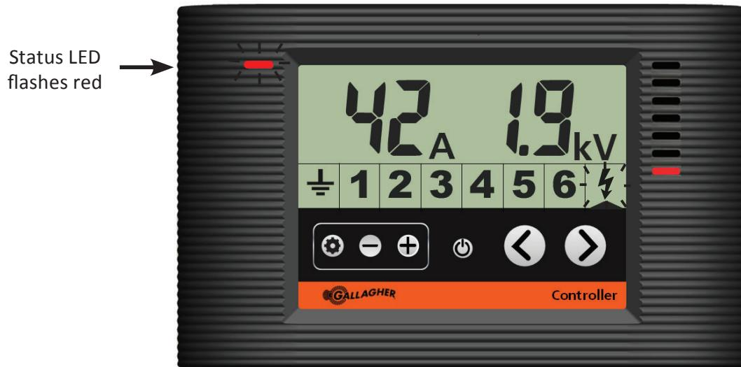
Controller showing the energizer in current alarm
