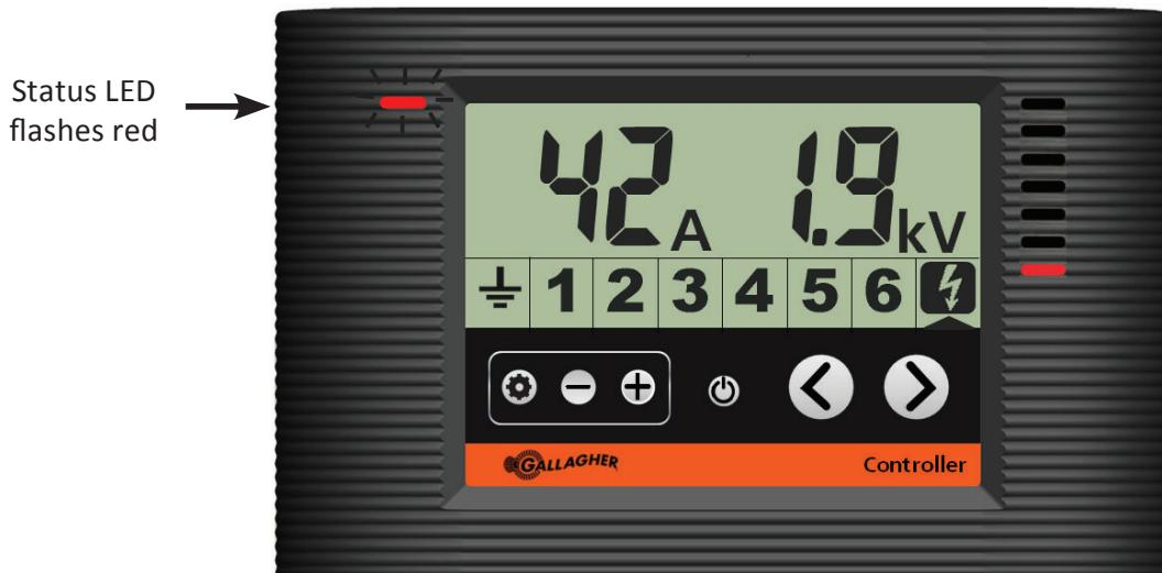
Controller showing the energizer in output alarm
