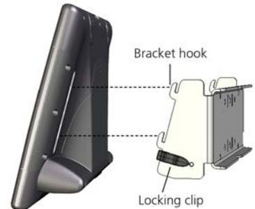
Attach the SmartTSi to the bracket
