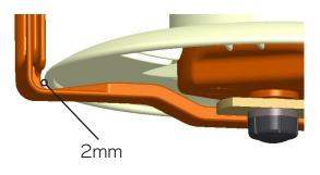
3. Clearance between wire guide and reel to be equal on both sides.
