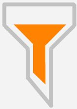
This icon displays when the time set for filter replacement has expired. Refer to *Tank Filter Replacement Timer on page 14*.
