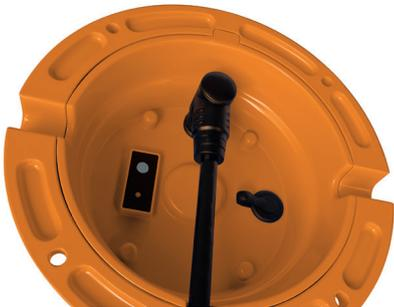
2. Wind the connector in a clockwise direction until it clicks securely in place, this ensures the required weather resistance.
