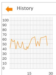
Touch the tank percentage icon on the main screen to display the HISTORY graph. This graph displays the recorded tank level for the preceding 30 days. Touch the centre of the graph to scroll through the different tanks connected to your system.
