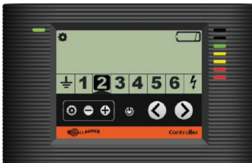
Controller showing zone 2 with a low battery
