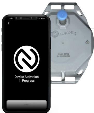
**5** During the activation the app will show 'Device Activation in Progress', ensure the back of your phone touches the device and is kept in the same position, for 10-30 seconds.
